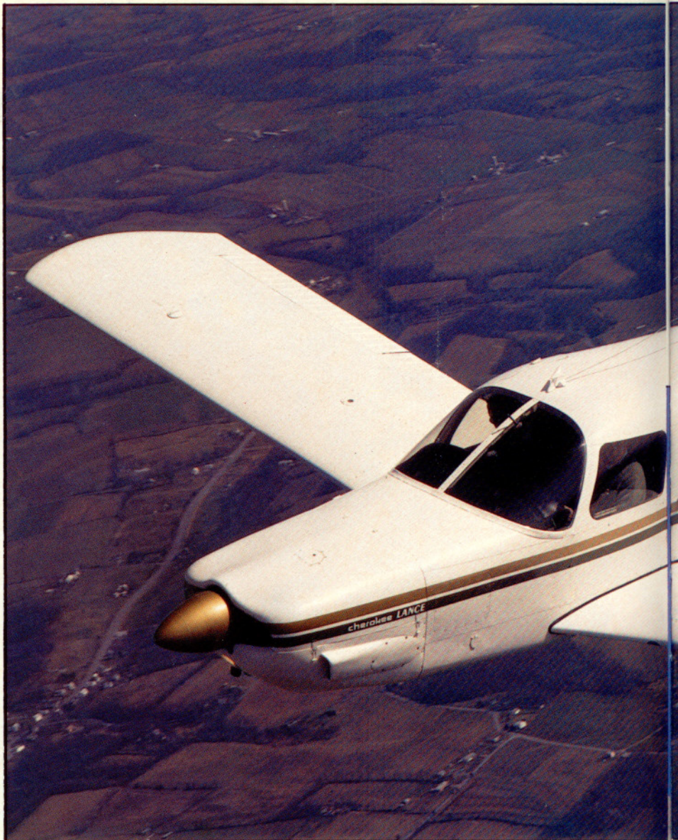
Not all Lances have T-tails. The original model lasted three years before "jet-age technology" struck.
