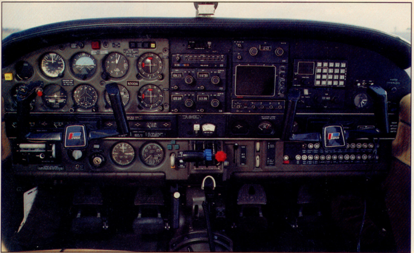
Mission-capable, this Turbo Lance is equipped with a hot prop, two-axis autopilot, weather radar, Loran receiver, engine-temperature monitor, fuel totalizer and standby electrical system.
